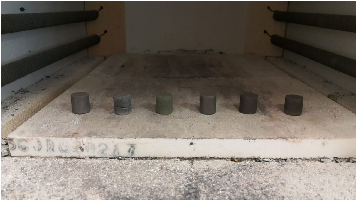
Fig. 1 Vertical cylinders in the furnace
