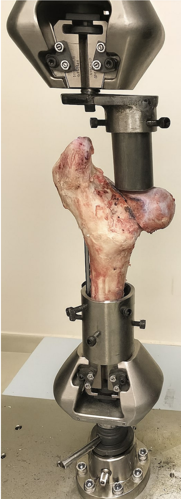
Figure 3. An axial compression test was performed on a bovine femur with a femoral neck fracture created and stabilized with dynamic hip screw using a Shimadzu AG-X 100 kN tensile testing machine.
